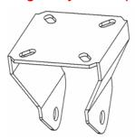
The bracket is made by an electrolytically galvanised steel fork.
