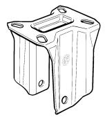
The bracket is made by a yellow galvanised steel fork.
