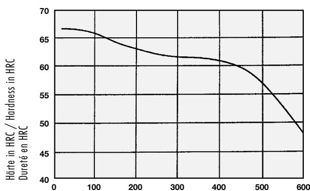
Anlasstemperatur in °C / Tempering temperature in °C
