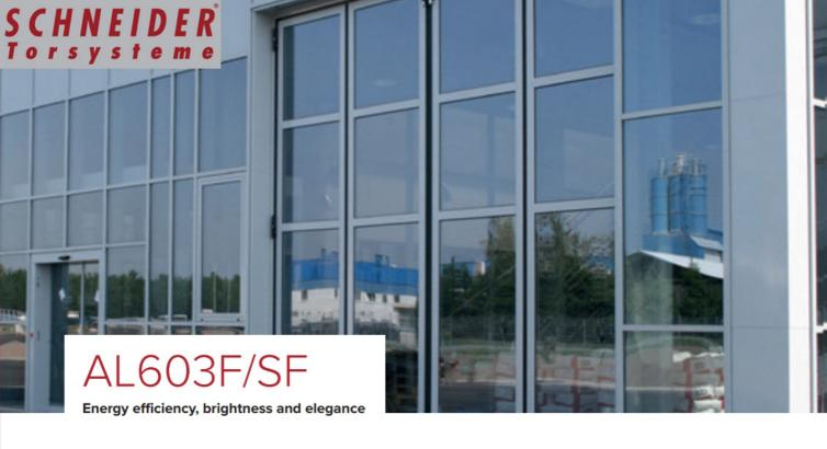
The innovative SCHNEIDER aluminium folding door AL603F/SF consists of specifically developed thermally separated profiles, which result in a substantially better thermal insulation than with normal profiles. The AL603F/SF profiles are connected using a screw-/plug-type system, forming a door with high torsional stiffness. As with the AL602F/SF, solid running rails, hinges and corner connections enhance the high load capacity and thus also enable large glass panels.
