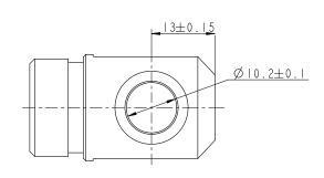
Option "D" and "E" Piston 0301244 with bushings, Stainless steel AISI 304 Piston 031923 with bushings, Stainless steel AISI 303
