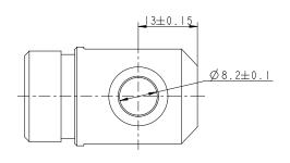
Option "6" Piston 0231016 with bushings, Zinc coated steel
