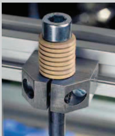
Picture 35.1: Polysorb disc springs in a fatigue test
