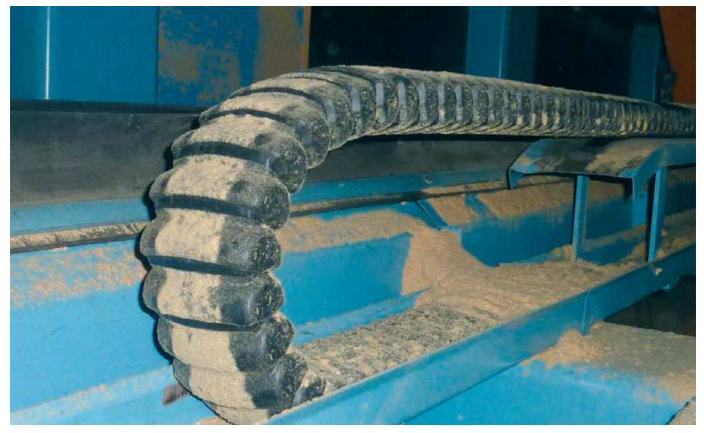
With the extremely chip-tight igus® RX e-tube and the harnessed chainflex® cables, the lifetime of this woodworking machine was considerably increased. Because of dust and dirt, previous cables failed after one month
