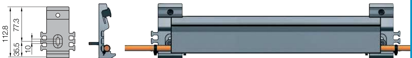
Version 01 - short trough bracket Part No. GF9.2.12 with integrated strain relief, \pm 5 mm vertical adjustment (electrically conductive version: GF9.2.12.CD)
