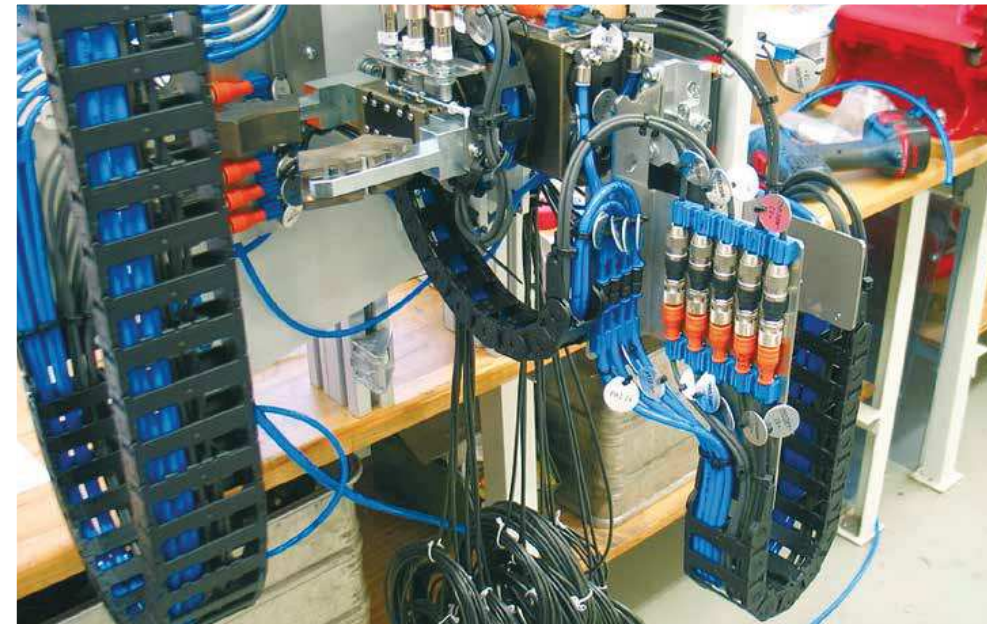
Strong and space-saving E2/000 e-chain® for different axes of a machine
