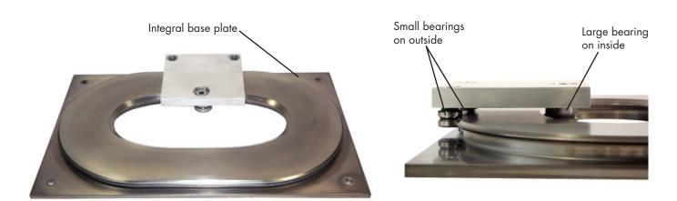
A further useful version of PRT2 1-Trak is shown below. In this design, the carriage fits inside a channel-section track which has inward-facing Vees that engage with the bearings. The advantage of this configuration is that the contact points between bearings and slide vees are spaced very far apart, giving higher moment load capacity and stiffness.
