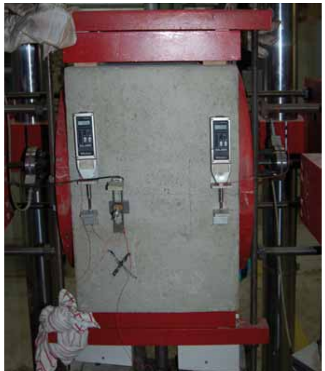
Test setup for cyclic load test
