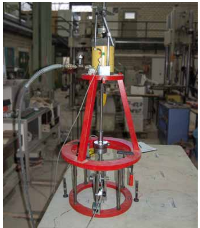
Test setup pull out tests
