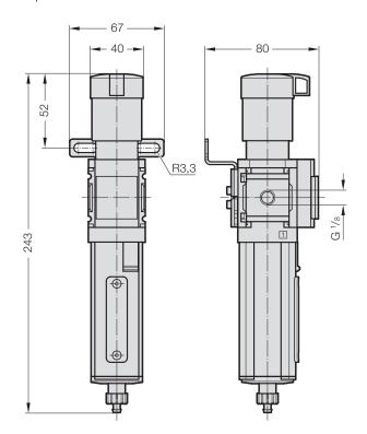
Compressed air maintenance unit for cleaning and regulating the control air of the cartridge valve in the active gas spring.
