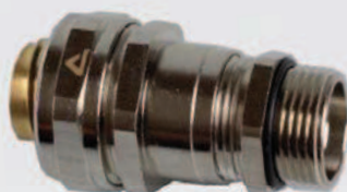
ISO cable-hose fitting, compact, male, nickel plated brass, double seal according EN 45545-2, HL1 / HL2 / HL 3, table R22 and R23 (incl. connection set).
