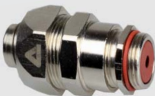
ISO cable-hose fitting, male, nickel plated brass, silicone clamping rubber up to max +220 °C (including connection set)
