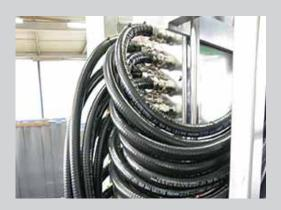
Anti-Static performance: Surface resistance < 10<sup>9</sup> Ohm, meeting the requirements of standard EN 60079-0, section 26.13
